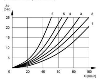
Refer to curve 5 for the pressure drops between working lines A and B of the spools S10, S20, S21, S22 and S23 used in regenerative schemes.
