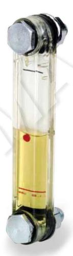
Thermoplastic level gauges made from transparent polyamide which provides good mechanical resistance and is impervious to mineral oil, gasoline, lubricants, petroleum, solvents and most chemical agents (please refer to technnical table N.1 page 58); avoid contact with alcohol based solutions and antifreeze liquids at high temperatures and hot water over 80°C
