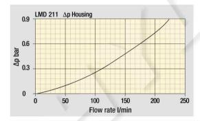
Bypass valve pressure drop
