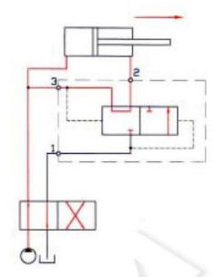
ration. Designed as an in-line valve, the SV-040 can be placed right at the cylinder ensuring the lowest possible pressure drop.
