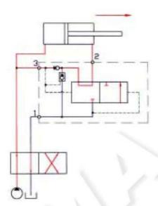
The Speed-Valve SVA-050 has a unique built in control valve, which automatically connects the rod side of the cylinder to tank when the cylinder meets resistance in the forward direction. This means the SVA-050 combines high flow and full force.
